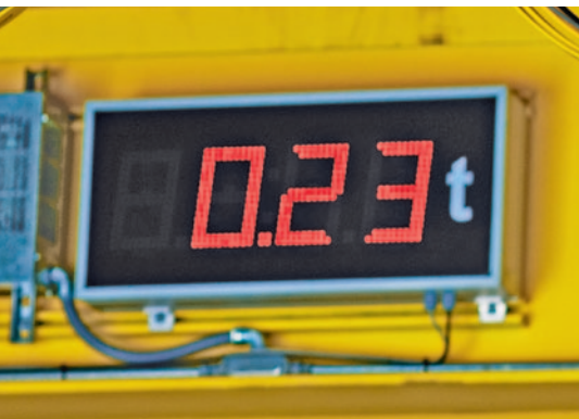
With large-format four-figure load summation for monitoring the total load on both hooks.
